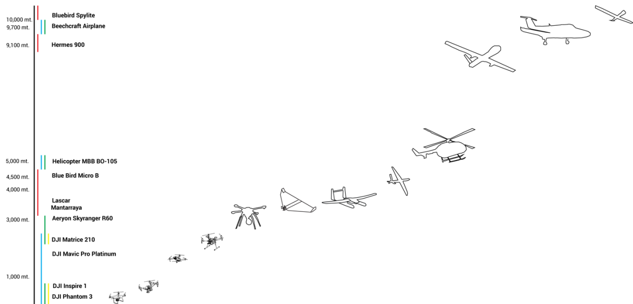
Figure 21 Diagram of aerial remote sensing systems of state and citizen security forces in Chile. Municipalities (yellow), Carabineros (green), PDI (blue), and Military Forces (red). Missing in this diagram is the Fasat Charlie satellite orbiting around the earth at 620 km (low earth orbit), obtaining high resolution multispectral images. The scale of drones is not strictly proportional. Another drone that may be owned by the state is the Elbit Skylark. The information I found was not clear on that case so I did not include it in the diagram. Finally, there are a myriad of drone prototypes built by the Chilean Air Force that I did not include as I don't know about their current operability and I did not receive any information on their uses 60 . Sources: interviews, promotional videos, press publications, and acquisition documents. (Josefina Buschmann, 2019)
